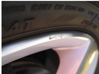
Non-chargeable wheel damage is defined as light scratches or scuffing that does not go through the paint or clear coat to the base material and may be removed with light sanding. This minor damage may cover up to 1/3 of the wheels circumference.
